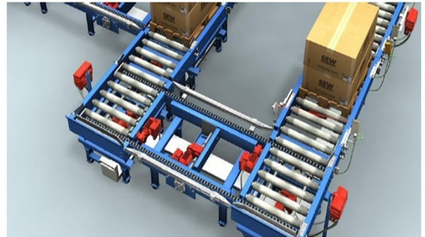
Fig. 1. Example of a Decentralized Installation Topology.
